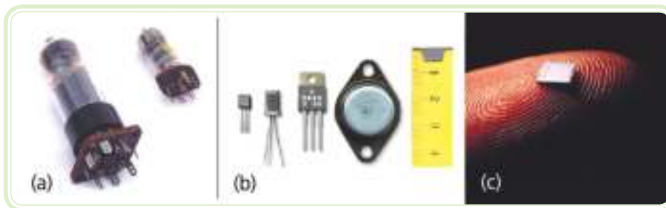
Figura 1.7: Válvulas (a), transistores (b) e microchip (c)
